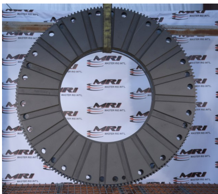
1320 Drawworks National 619296 - Center Plate, 36 C 619295 - Plate, 36 Air
